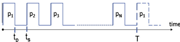
Fig. 2. Schematic of the polyphase excitation sequence. The duration of each pulse is t_p , and the entire sequence is repeated cyclically with period T . The time between the start of two successive pulses is t_s , so t_s N = T . Phases p_1, \dots, p_N are the elements of the Frank sequence.
